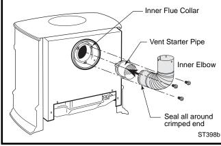
Fig. 22 Install inner starter pipe and inner elbow.
